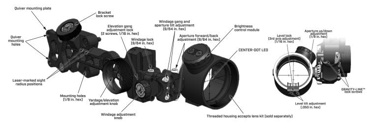
**NOTE:** The detachable/adjustable bracket model (AG2301BD) is shown. On standard bracket models, all adjustments are the same, excluding the bracket lock screw and the quiver mounting plate. The standard bracket includes multiple sight radius mounting positions and the quiver can be mounted to the sight without an extra mounting plate.
