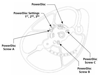
Figure 3: PowerDisc Adjustment
