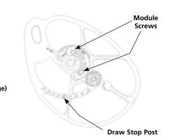
BT-X 28" Cam Module Draw Post Position Length Setting 28 1 1 2 27.5 2 27 3 3 4 26.5 4 5 26 5 25.5 6 6
