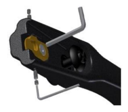
The alignment of the limbs can be done with **bow unloaded**, operating the two side grains, after removing the two locking grains and slightly loosening the central screw. When alignment is done, tighten the grain on the opposite side of where you last worked, re-insert and tighten the locking grains and the central screw.
