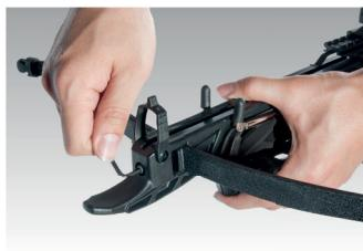
**1.EN:** Insert prod into stock to the white line. Make sure the pressure pad is in place between the prod and the prod retaining screw. Do not over tighten.
